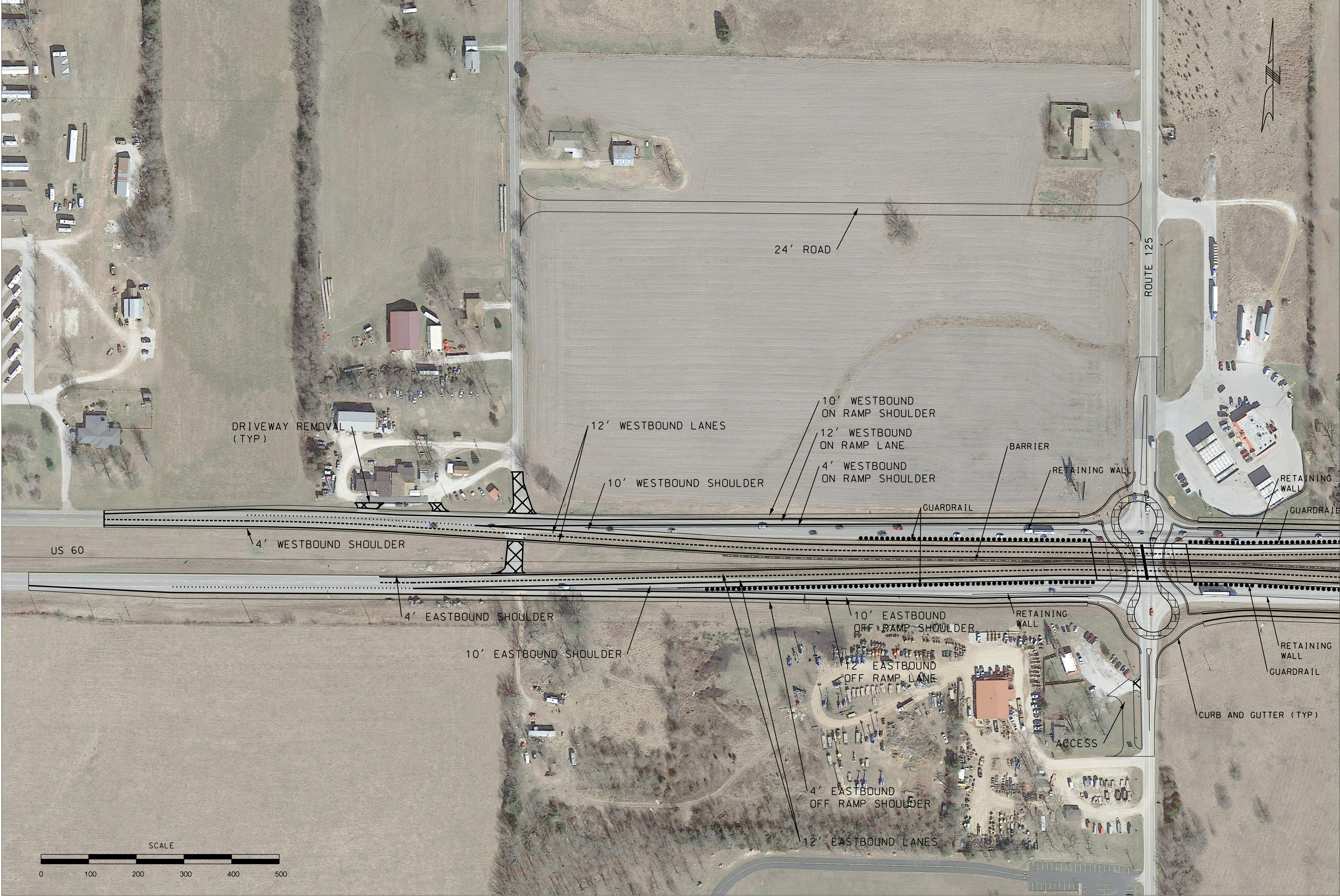
J8P0683E / US-60 - ROUTE 125 INTERCHANGE
