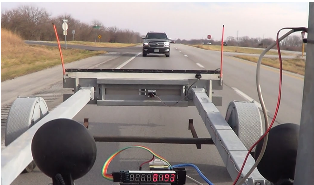
Figure 4. The distance of vehicles from the rear-advance TMA were measured using a LiDAR detector.
